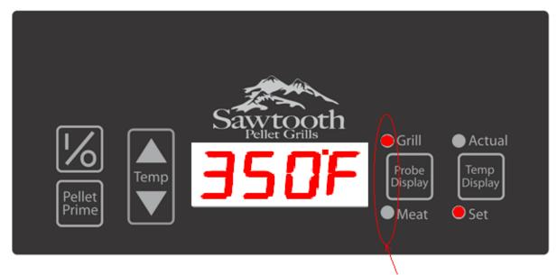
Note that if the Ignitor is on, the LED lit in this column will blink.
