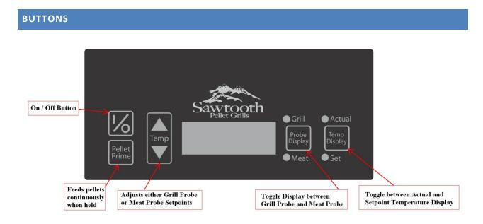
Probe Display – Toggle Display between Grill Probe and Meat Probe
