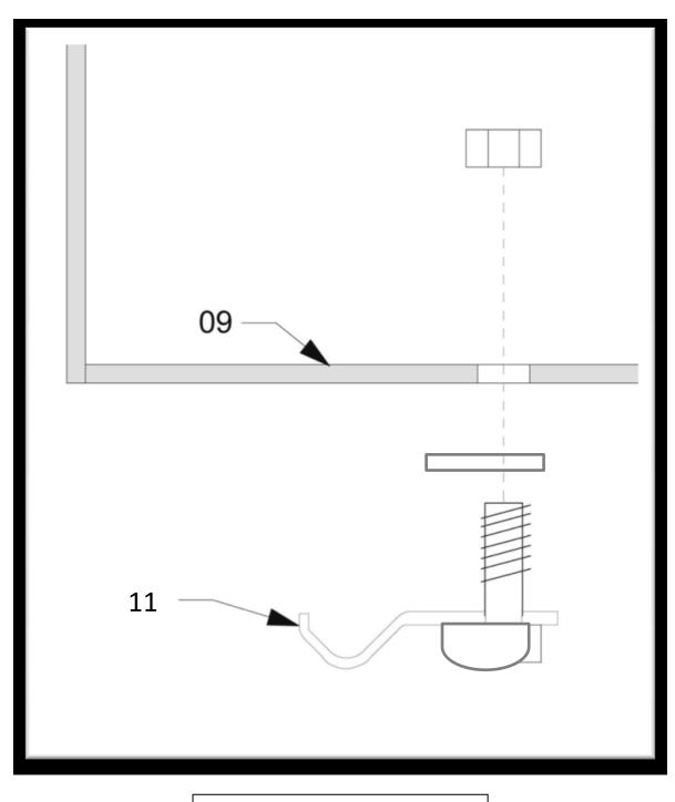
Tools – 7/16 Open end wrench & Phillips screw driver Place the Phillips headed bolt with washer through the bracket and the grill. Then apply the nut to the top and tighten.
