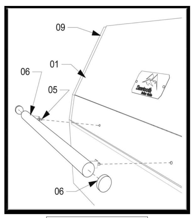
Tools – 7/16 Open end Wrench & Phillips screw driver Place a plastic grommet in the end of each side of the handle and press them in. Place the Phillips head bolts through the pre drilled holes in the handle and the lid. Place a nut on the back of each bolt and tighten until snug.
