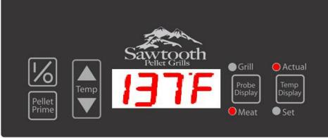
In this state, if the Temp Up or Down buttons are pressed, the display will revert to the Meat Probe Setpoint Display state.
