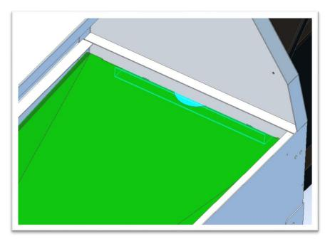
Install drip tray with notch at right side of grill. Bottom flange on drip tray will rest on drip tray rest at right (above). The left side of drip tray will rest in the grease catch tray at the left of the grill (below). Drip tray should be evenly space from front to back. Take care not to block air flow around sides of drip tray.
